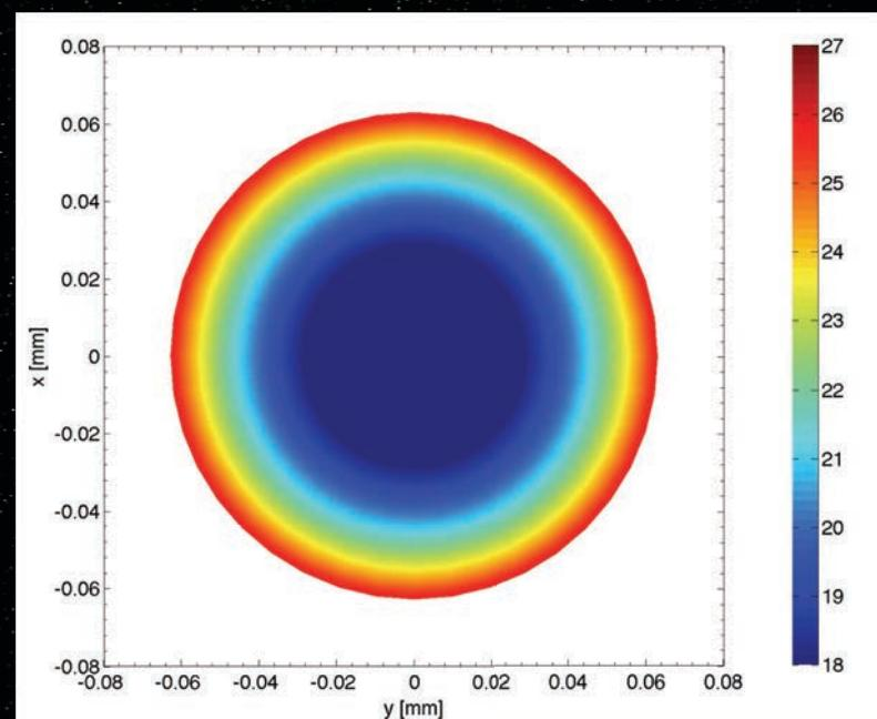
Temperature gradient on the SODISM front window
