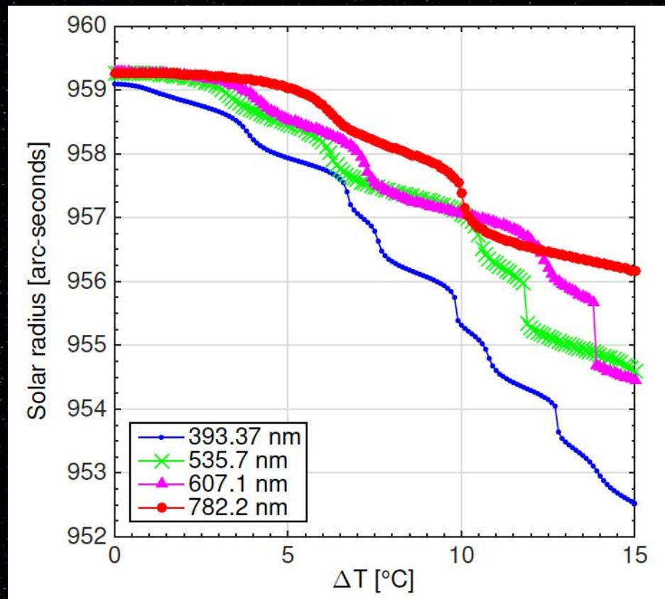
Evolution of the solar radius (determined by the inflection point position method) as a function of a temperature gradient for different wavelengths.
