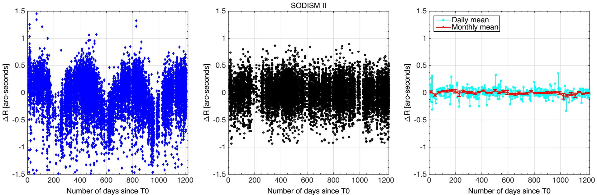
(Left) Evolution of the solar radii at one astronomical unit (uncorrected and corrected data for refraction with mean value of  $k$ ) since the first measurements carried out by SODISM II in May 2011.
