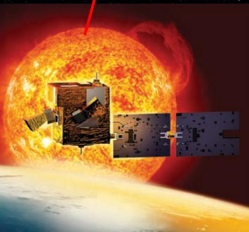
**PICARD** is a space-based mission, which was launched on 15 June 2010 into a Sun synchronous dawn-dusk orbit (735 km, Inclination: 98.29°).
